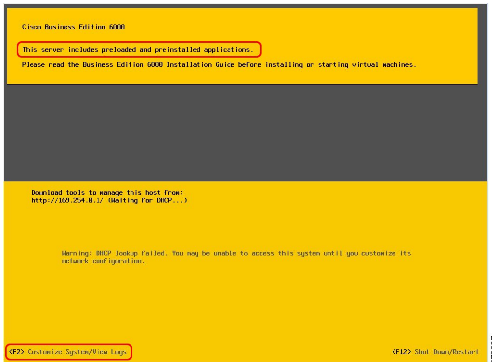
Figure 3: Console Screen After ESXi Loads
