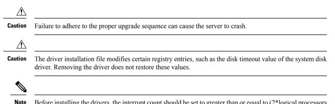
Before installing the drivers, the interrupt count should be set to greater than or equal to (2\*logical processors + 4) for VIC 14XX adapters. The interrupt value can be rounded up to the nearest second power. For more information on how to set the interrupt field for Ethernet adapter policies in the UCS Manager GUI, refer to the UCSM Network Management Guide.
