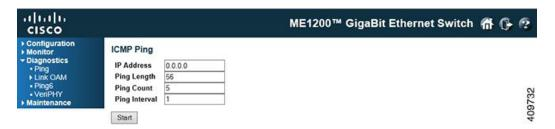
After you the press **Start** button, ICMP packets are transmitted, and the sequence number and round trip time are displayed upon reception of a reply. The amount of data received inside of an IP packet of type ICMP ECHO\_REPLY will always be 8 bytes more than the requested data space(the ICMP header). The page refreshes automatically until responses to all packets are received, or until a timeout occurs.
