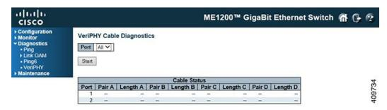
Press the **Start** button to run the diagnostics. This will take approximately 5 seconds. If all ports are selected, this can take approximately 15 seconds. When completed, the page refreshes automatically, and you can view the cable diagnostics results in the cable status table. Note that VeriPHY is only accurate for cables of length 7 - 140 meters.
