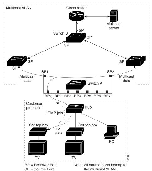
These messages dynamically register for streams of multicast traffic in the multicast VLAN on the Layer 3 device. Switch B. The access layer switch, Switch A, modifies the forwarding behavior to allow the traffic to be forwarded from the multicast VLAN to the subscriber port in a different VLAN, selectively allowing traffic to cross between two VLANs.
