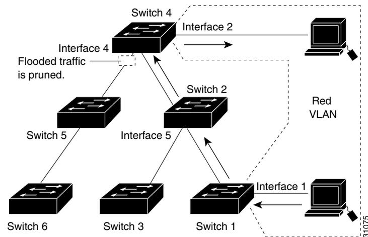
Enabling VTP pruning on a VTP server enables pruning for the entire management domain. VTP pruning takes effect several seconds after you enable it. By default, VLANs 2 through 1000 are eligible for pruning. VTP pruning does not prune traffic from pruning-eligible VLANs. VLAN 1 is always ineligible for pruning; traffic from VLAN 1 cannot be pruned.
