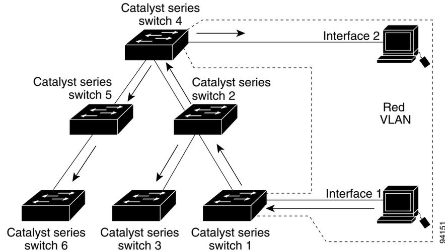
Figure 13-3 shows the same switched network with VTP pruning enabled. The broadcast traffic from Switch 1 is not forwarded to Switches 3, 5, and 6 because traffic for the Red VLAN has been pruned on the links indicated (Interface 5 on Switch 2 and Interface 4 on Switch 4).
