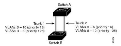
Trunk 1 carries traffic for VLANs 8 through 10, and Trunk 2 carries traffic for VLANs 3 through 6. If the active trunk fails, the trunk with the lower priority takes over and carries the traffic for all of the VLANs. No duplication of traffic occurs over any trunk port.
