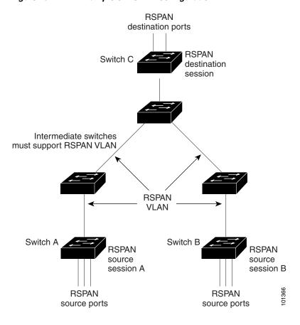
Figure 23-2 Example of RSPAN Configuration
