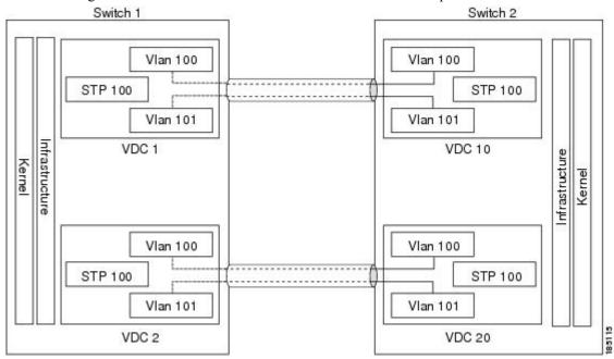
Each VDC acts as a standalone device with Layer 2 services available. VDCs allow you to share a physical device among several logical functions. You can provision and assign entirely separate Layer 2 resources to individual VDCs.
