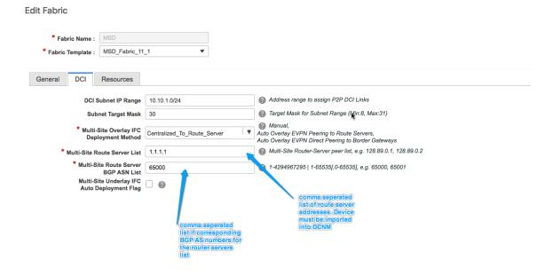
The IFCs needed for deployment of Networks and VRFs at the BGW nodes can be auto configured via the MSD fabric template. The settings to enable that are in MSD fabric template.
