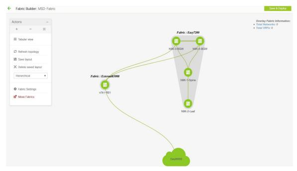
VXLAN BGP EVPN intra-fabric configurations, including network and VRF configurations are provisioned on the switches through DCNM software, 11.1(1) release. However, server traffic between the fabrics is only possible through the following configurations:
