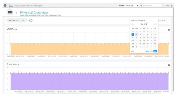
**3.** Hover over specific points on the respective graphs to display the number of VPC peers and Transceivers that are associated with a switch at a specific time.
