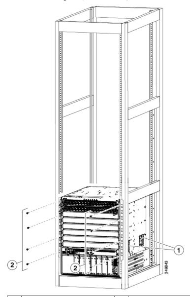
Handles used to adjust the chassis 2 placement.
