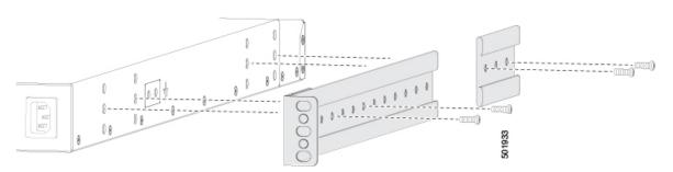
c) Secure the front-mount bracket and the back-mount bracket to the chassis using four M4 screws and tighten each screw to 12 in-lb (1.36 N·m) of torque.
