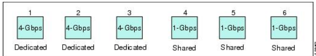
Figure 8: Example Speed and Rate Configuration on a 24-Port 4-Gbps Switching Module
