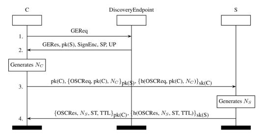
**Figure 4.** Sequence diagram showing the procedure for establishing a secure channel within the UA-SecureConversation protocol [3]
