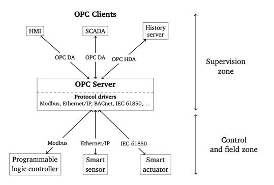
Figure 1. Example deployment of an OPC solution within an industrial system
