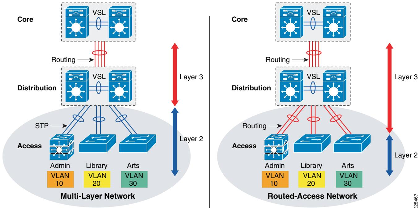
At the network edge, Layer 3 access switches provides an IP gateway function and becomes a Layer-2 demarcation point to locally connected endpoints that could be logically segmented in multiple VLANs.
