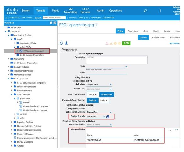
The figure shows that a device at IP address 192.168.103.21 has been quarantined.
