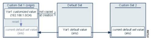
This approach adds Var1 to all sets with a default value of any. After adding Var1, you can customize its value in any set. An advantage of this approach is that, by not initially customizing Var1 in the default set,
