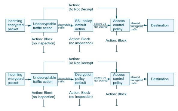
A more complex SSL policy can handle different types of undecryptable traffic with different actions, control traffic based on whether a certificate authority (CA) issued or trusts the encryption certificate, and use TLS/SSL rules to exert granular control over encrypted traffic logging and handling. These rules can be simple or complex, matching and inspecting encrypted traffic using multiple criteria.
