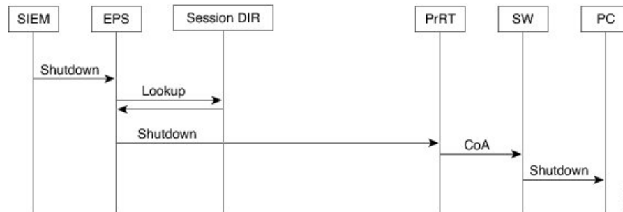
Figure 2: EPS ANC Shutdown Flow
