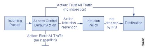
The following table describes how the different default actions handle traffic, and lists the types of inspection you can perform on traffic handled by each default action. Note that you **cannot** perform file or malware inspection on traffic handled by the default action. For more information, see Controlling Traffic Using Intrusion and File Policies, page 10-1.
