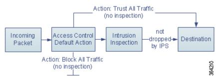
Note that only ASA FirePOWER modules deployed inline can affect the flow of traffic. Applying an access control policy configured to block or alter traffic to passively deployed devices can have unexpected results. In some cases, the system prevents you from applying inline configurations to passively deployed ASA FirePOWER modules.
