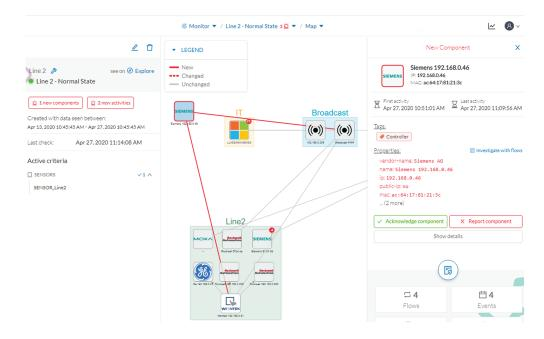
Then, we check that this new component behaves normally by looking at its activities. It has been identified because it has sent a broadcast packet (probably ARP) and then has connected to the Weintek machine using a legitimate protocol. Actions like Read variable accesses look normal too.
