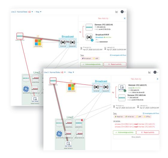
Since the component and activities will be part of the normal operating process of Production Line 2, the differences can be acknowledged and included in the baseline to be notified if any change occurs.
