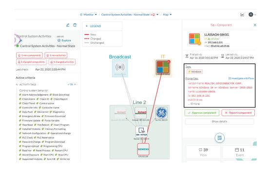
Clicking the new activity between the new machine and the CPU opens its right side panel and gives more information about what happened. New tags such as Firmware Download, Start CPU, Stop CPU, Read and Write Var, which are suspicious, indicate the type of actions the new Windows machine has performed on the CPU.
