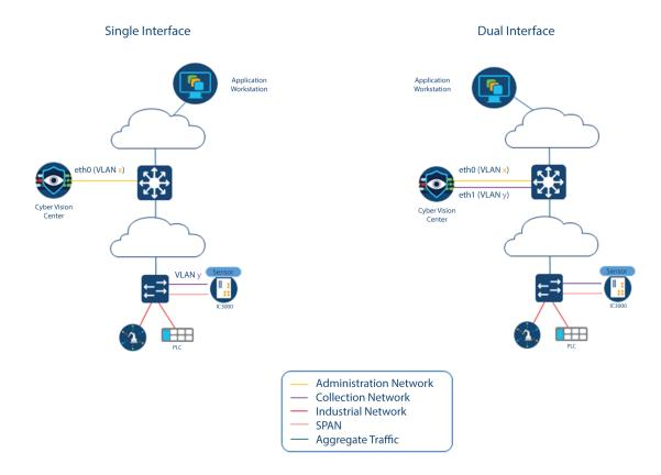
The Center provides two dedicated and separate 10 Gigabit Ethernet network ports to connect to these two networks.
