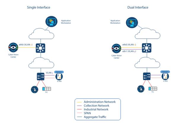
The Center provides two dedicated and separate 10 Gigabit Ethernet network ports to connect to these two networks.
