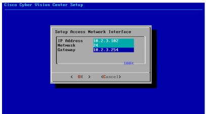
Enter the Administration network interface's IP address, netmask (in a two-number format), and gateway.
