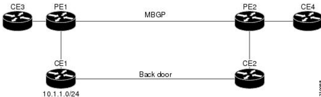
Figure 2: Network Showing How Cost Community Can be Used to Support Backdoor Links
