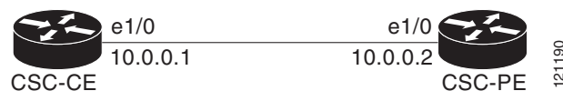
Figure 37 Configuration for Peering with Directly Connected Interfaces Between CSC-PE and CSC-CE Routers
