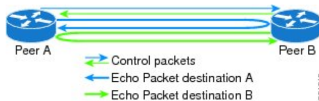
Figure 9: BFD Asynchronous Mode With Echo Packets
