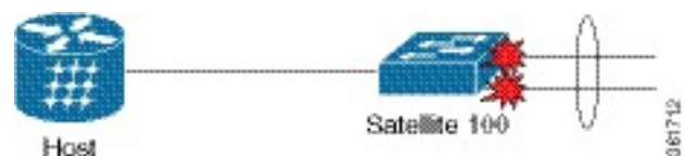
Figure 11: Service-policy on Access Port over Bundle Interface
