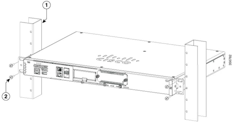
Figure 4: Mounting the Chassis on the Rack – I/O-Side (Cisco 8200 Series Chassis)
