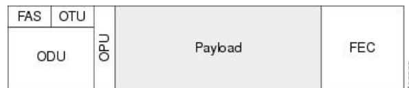
Figure 1: OTN Optical Channel Structure
