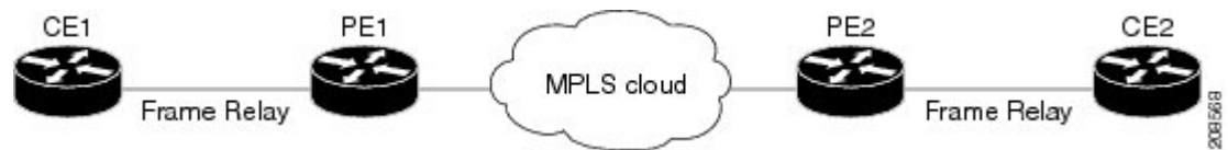
Figure 8: Frame Relay Over MPLS
