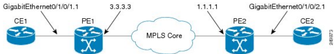
Figure 38: VPLS with BGP autodiscovery and BGP signaling
