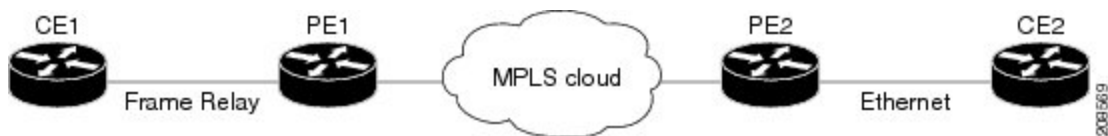
Figure 9: IP Interworking Over MPLS
