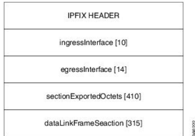
Figure 4: IPFIX 315 Export Packet Format
