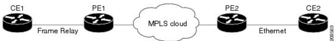
Figure 2: IP Interworking Over MPLS
