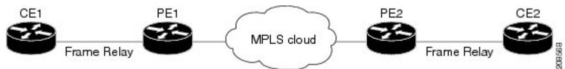
Figure 1: Frame Relay Over MPLS
