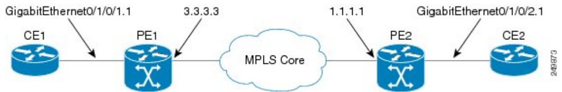
Figure 20: VPLS with BGP autodiscovery and BGP signaling
