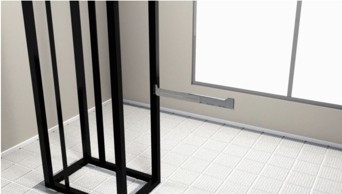
Figure 13: Four Post Slider Integration in the 23" Rack
