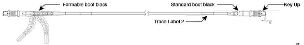
Figure 2: Cable with Formable Boot and Standard Boot
