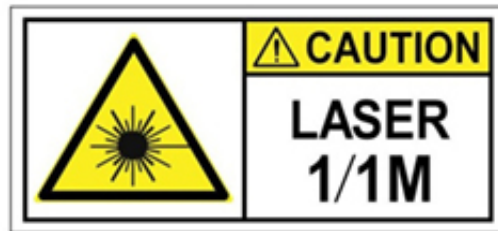
Figure 19: Class 1M Laser Product Label
