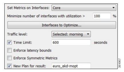
The tool tries to find the most optimal solution it can. In general, the longer it runs, the better the result. The Time Limit option tells the tool to stop looking for better solutions after the specified amount of time, and use the best solution it has found so far. If the option is not set, the tool continues to run until it runs out of solutions to explore, which can take a long time. If you need all available solutions to be explored, use the Metric Optimization, on page 2 tool.
