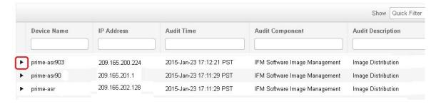
**Step 2** Expand an event drawer to get details about a device change. For example, if you expand the drawer highlighted in the above figure, you can see that the image listed in the job was successfully distributed to the device.
