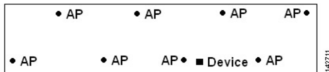
Figure 4: Improved Location Accuracy by Staggering Around Perimeter
