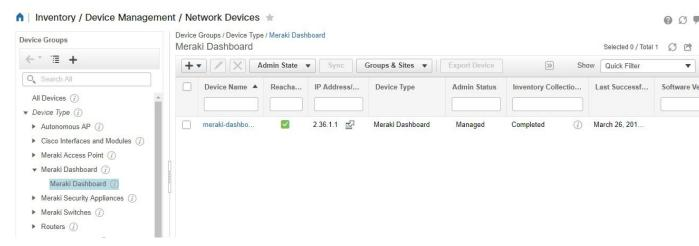
The Meraki Dashboard remains the single point of configuration for Meraki devices. Cisco Prime makes it very easy to get to any specific device by including a device link next to the IP Address of the device. These links will launch a browser window that will bring the administrator right to the device in the Meraki Dashboard which helps you to extract comprehensive information about a particular device.
