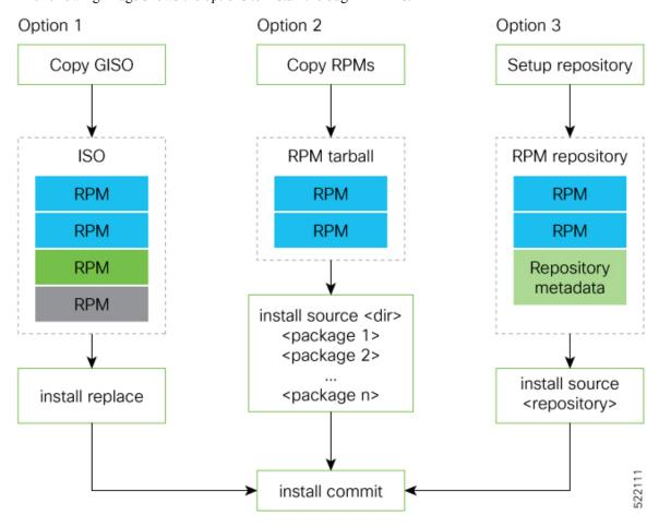
The software is split into modular blocks and the package manager infrastructure computes the dependencies between the blocks. Each block of software has a top-level package and various partition-level packages. Bug fixes that span multiple blocks may lead to creating multiple dependent packages that are built as part of earlier bug fixes.
