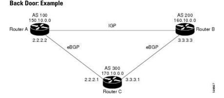
Here, Routers A and C and Routers B and C are running eBGP. Routers A and B are running an IGP (such as Routing Information Protocol [RIP], Interior Gateway Routing Protocol [IGRP], Enhanced IGRP, or Open Shortest Path First [OSPF]). The default distances for RIP, IGRP, Enhanced IGRP, and OSPF are 120, 100, 90, and 110, respectively. All these distances are higher than the default distance of eBGP, which is 20. Usually, the route with the lowest distance is preferred.
