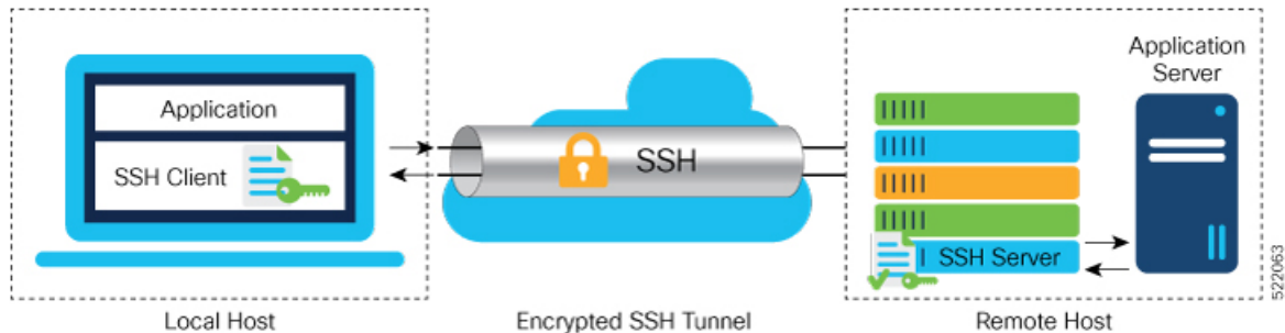
Figure 1: SSH Port Forwarding
