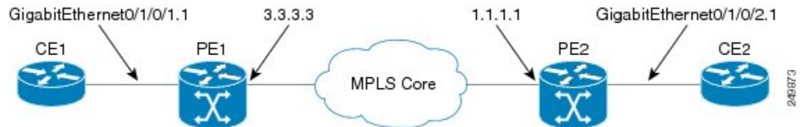
Figure 10: VPWS with BGP autodiscovery and LDP signaling
