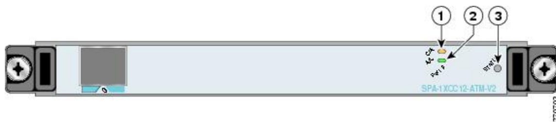
Figure 33: 1-Port Clear Channel OC-12 ATM SPA Faceplate
