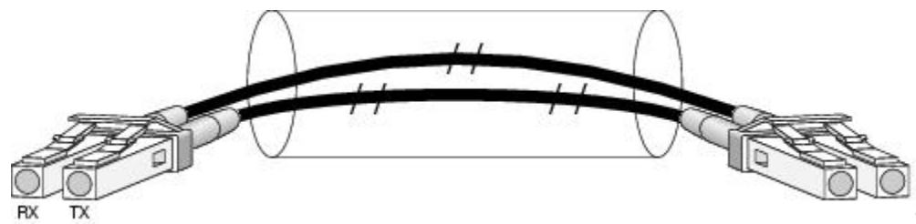
Figure 14: LC-Type Cable for the XFP Optical Transceiver Modules
