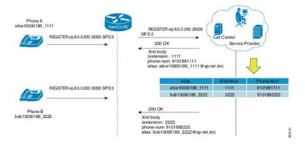
The AOR sent in the REGISTER is an alias which is mapped to an extension and/or phone number by the service provider. The service provider returns the mapping details in the 200 OK response sent to the REGISTER. Nano CUBE provides the ability to cache the alias mapping details in its call routing database. When a call is made from the phone, the Request-URI of the INVITE contains the dialed number (short extension or phone number).
