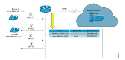
Earlier, when WAN was down, User A could only contact User B using either the alias or the user-id of User B, and not using their extensions or phone numbers.
