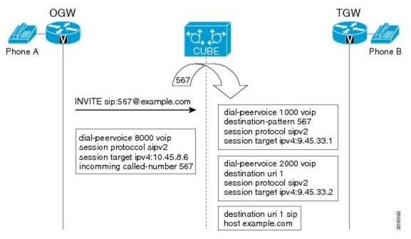
With the introduction of the domain-based routing feature, all parameters including the domain name of the request URI will be sent to the application and the outbound dial peer can be matched with any parameter. In Figure 1, when the domain name example.com is used to match an outbound dial peer the resulting dial peer is 2000. The **call route url** command is used for configuring domain-based routing.
