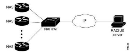
RADIUS servers normally check the source IP address in the IP header of the RADIUS packets to track the source of the RADIUS requests and to maintain security. The NAT or PAT solution satisfies these requirements because only a single source IP address is used even though RADIUS packets come from different NAS routers.
